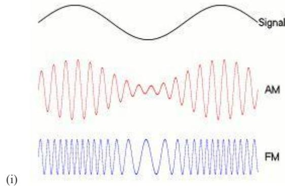
**Frequency range of working:** Amplitude modulation works between 540-1650 KHz while FM works at 88-108MHz.
